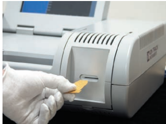
The reusable sample trap carries minute particles to the Itemiser.
