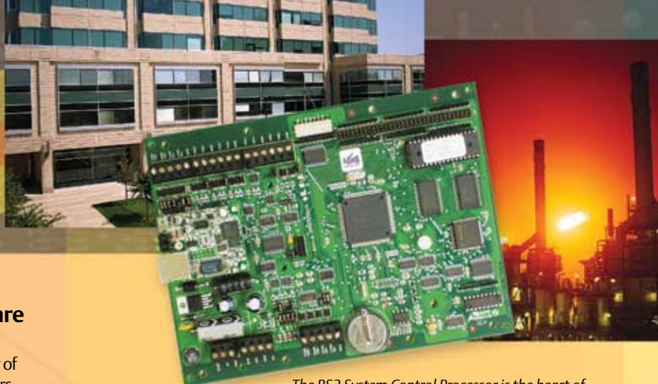
The RS2 System Control Processor is the heart of every RS2 access management system.
